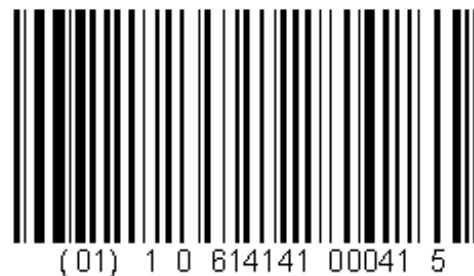
Shipping Container Code - UCC/EAN 128 format. Note: not actual size. The dotted lines indicate the location of the borders of the quiet zones.
